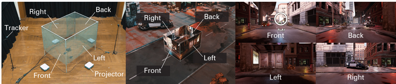
Figure 2: Relationships between four cameras and each screen for VR projection. Left: Setup of the ReverseCAVE with a cubic screen. Middle: Captured cubic image for projection (placed on the VR environment for explanation). Right: Rendered images for each screen plane.
